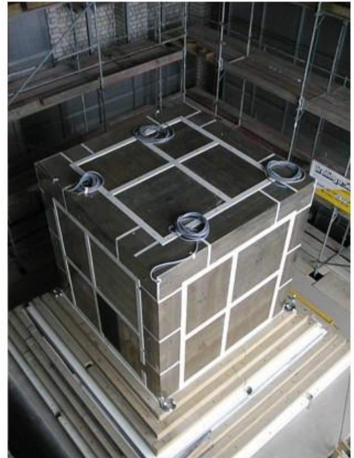
Figure 5: Photograph of the magnetic shield under construction, view on the top, the right wall and the rear wall of the inner cube with the first MUMETALL shell.
