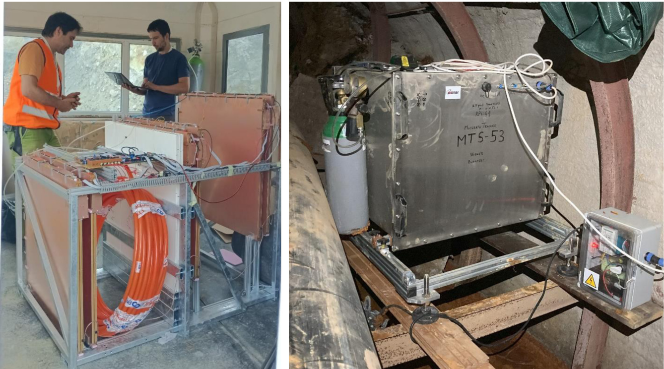
FIG. 8. The surface detector in a container (left) and the underground detector in the dewatering tunnel (right).
