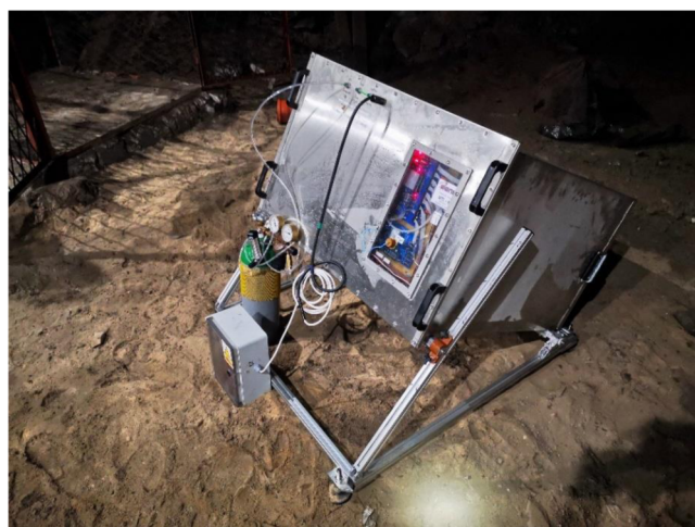
FIG. 1. An “Mti” type MWPC detector with stainless steel casing. In front of the detector, the gas system and the power box can be seen. The active size of the chambers is 80 \times 80 cm 2 .
