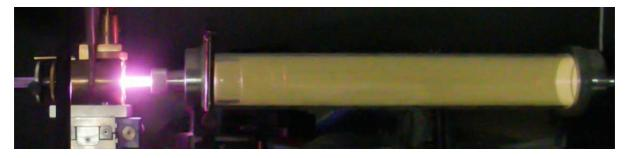
*Figure 5. Microwave surface-wave excited plasma (left, bright part), and reactive streaming afterglow (right, large volume part)*
