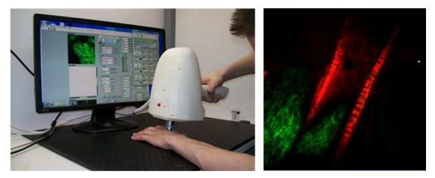
**Figure 2. Left:** Photo of our handhold nonlinear microscope system (FiberScope) developed for basal cell carcinoma detection. **Right:** Corresponding test image recorded for a murine skin sample at the properly set fiber laser wavelength (SHG and 2P)
