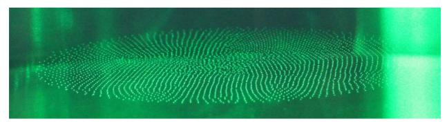
Figure 2. Image of a single layer dust cloud levitating in a gas discharge
