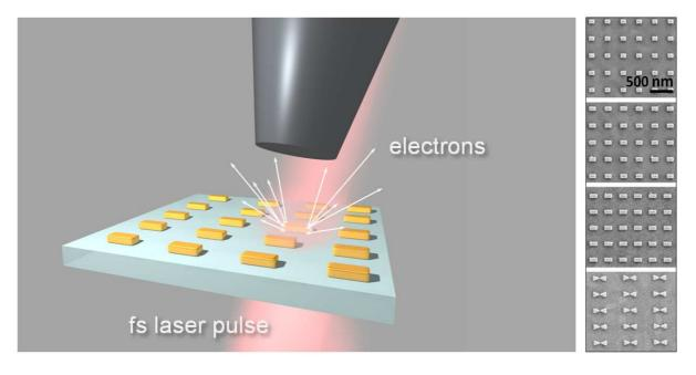
**Figure 1.** Experimental scheme on photoemission from metallic nanoparticles, including nanorods on a glass substrate. The illuminating femtosecond laser beam comes from below and the spectrometer tube collecting the electrons is also depicted. The different nanoparticles investigated are shown on the right-hand-side.
