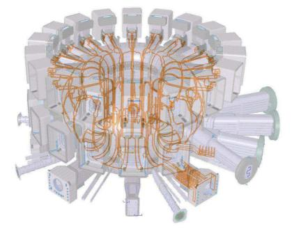
Figure 1. Component of TSD project (cables, cable trays, feedthroughs, connectors)
