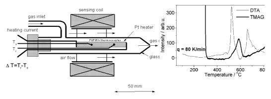
Fig.4. Probe head for DTA and TMAG measurements
