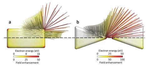
Fig. 1. Spatial distribution of electrons in photoemission from metallic nanoparticles, including (a) nanorods and (b) bowtie-type structures. The electron energy is encoded in the colour and length of the trajectories.
