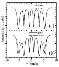
Fig.1. Simulation of reciprocity-obeying (a) and violating (b) arrangements in Mössbauer scattering [MR.1].
