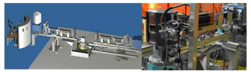
Figure 2. Layout of the GINA neutron reflectometer with the upgraded monochromator and slits
