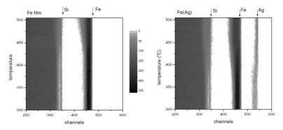
Fig. 1. Real-time BS measurements using 2000 keV<sup>4</sup>He<sup>+</sup>-beam on a 50 nm Fe film (left) and Fe film containing 1 at. % Ag (right) on Si(100) using ramped annealing (1.9 °C/min). Every horizontal line in such a contour plot corresponds to an RBS spectrum, with a tone scale representing the backscattering yield.
