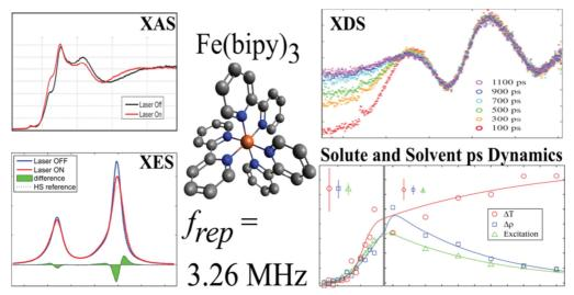
Fig. 1. Combined X-ray absorption and X-ray emission spectra, and X-ray diffuse scattering results that resolve a subnanosecond-lived excited Fe(II) state.
