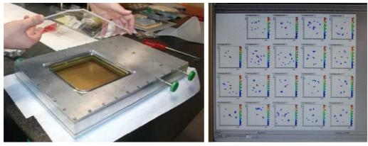
Fig. 1: ThickGEM-based photon detector during assembly
