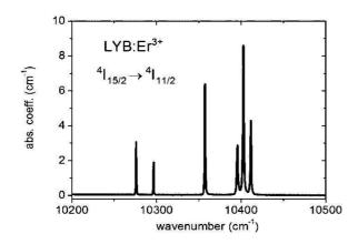
Fig.1. Crystal field splittings of the  ${}^{4}I_{11/2}$  level of  $Er^{3+}$ in  $Li_{6}Y(BO_{3})_{3}$  crystal at 8 K
