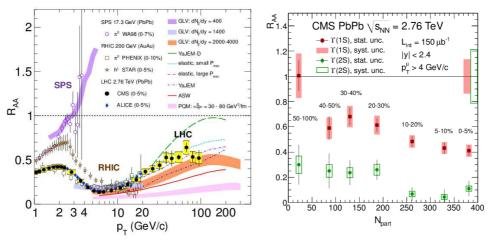
Fig 1. CMS: The nuclear modification factor  $R_{AA}$  in central heavy-ion collisions for neutral and charged hadrons, at several center-of-mass energies.
