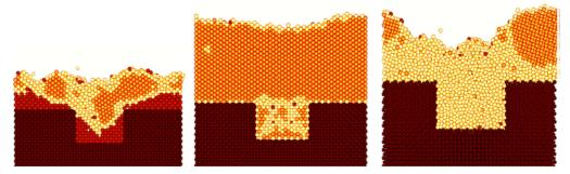
Fig. 1. Freezing on fcc substrate with a rectangular nanoscale pit. Spheres drawn around reduced density peaks larger than  $\Psi = 0.05$  are shown. Order parameters q4 and q6 are used
