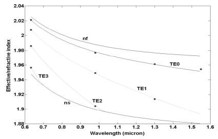
Fig.2. Multispectral reconstruction of the refractive index of the guiding and barrier layer as a function of the wavelength in a 3.5 MeV  $N^+$  ion irradiated planar waveguide in Er: Te glass. Sample was irradiated with  $8 \times 10^{16}$  ions/cm<sup>2</sup>. Calculated effective indices (nf and ns) of the modes are also shown.
