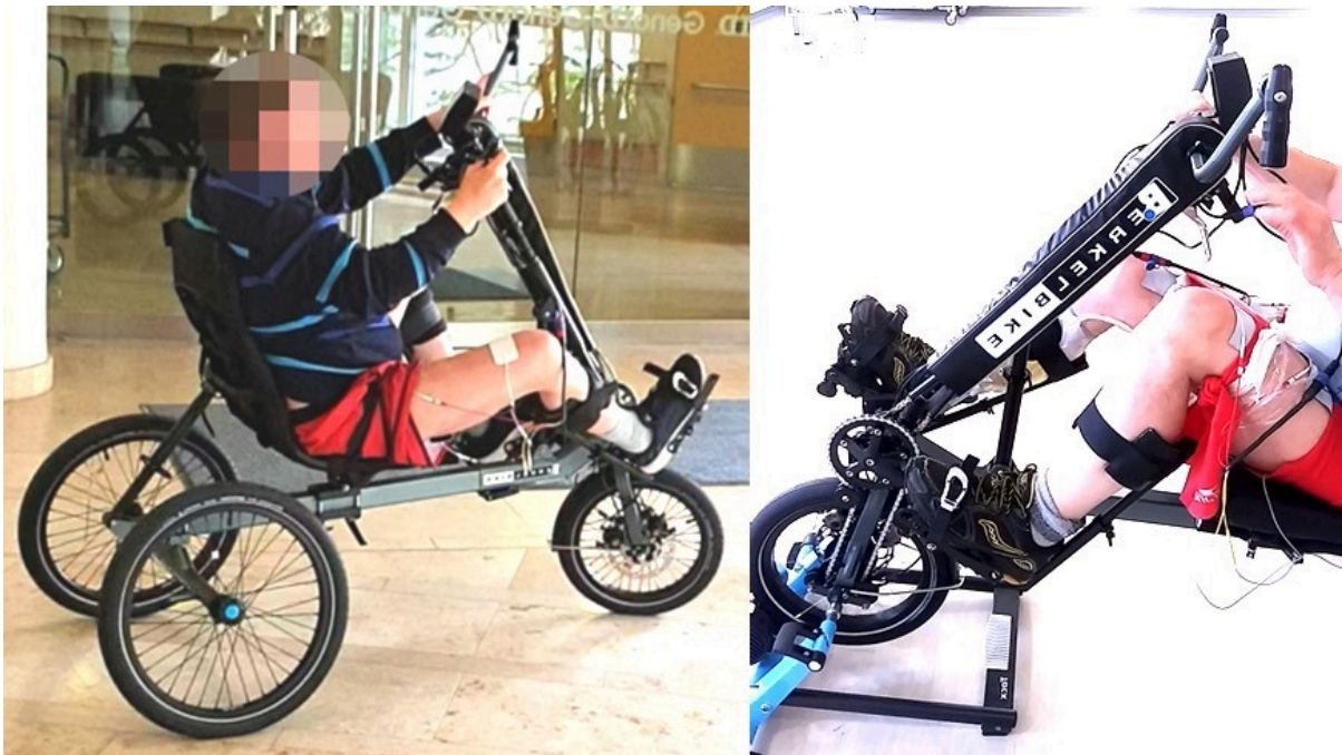
Figure 2. A person with spinal cord injury and paralyzed lower limbs, is "tricycling" on a Berkelbike tricycle. He propels the tricycle with his paralyzed limb using functional electrical muscle stimulation (FES). His leg muscles (quadriceps, hamstrings and gluteus maximus) exert active forces controlled by FES.
