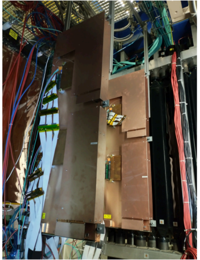
Figure 3 : The 120cm long GRC chamber for the CERN NA61 experiment: during construction (left) and inside the experiment after installation (right).
