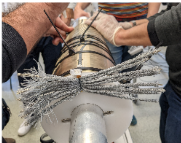
Fig. 4. Test winding of a straight CCT former for the HITRI+ project.
