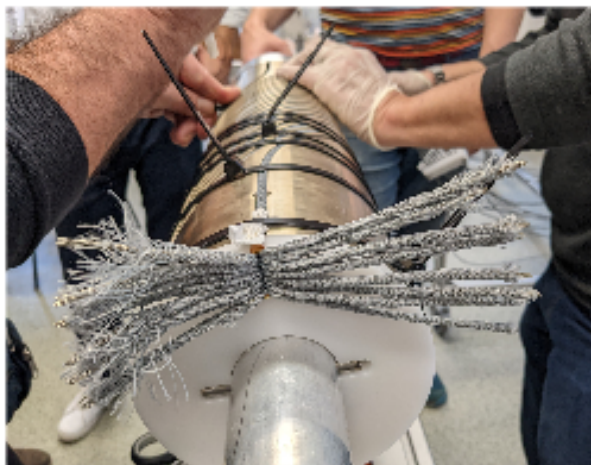
Fig. 3. Demonstration of the wax impregnation method. A single CCT layer impregnated with wax, without voids.
