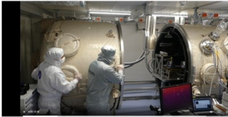
Figure 2. Closing the thermo vacuum chamber in Bern where PEP's operation was tested from -170^{\circ}\text{C} up to +60^{\circ}\text{C} in a duration of 4 weeks.
