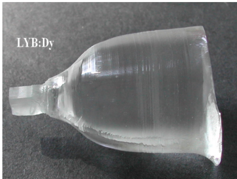
Figure 1. High optical quality LYB crystal doped with Dy.
