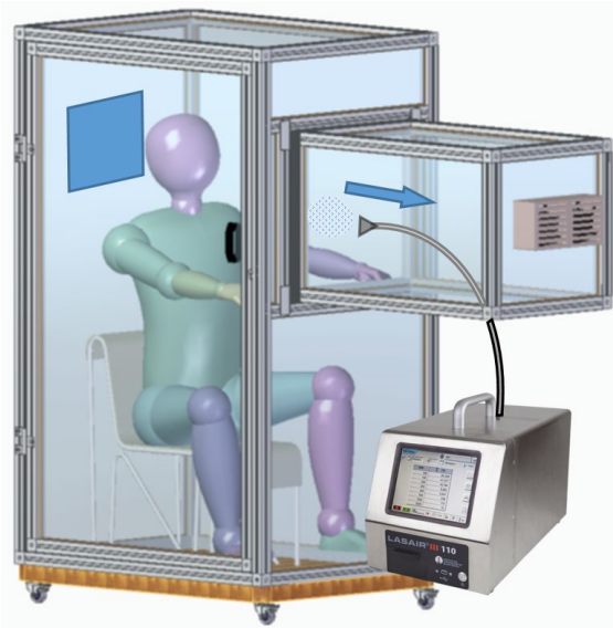
Figure 1. The measurement set-up (left panel) and typical size distributions of emitted particles during different activities (right panel). A weak laminar flow was maintained in the cabin through a ULPA filter to achieve cleanroom conditions. For the mask tests, subjects performed the same activity (counting from 1 to 100).
