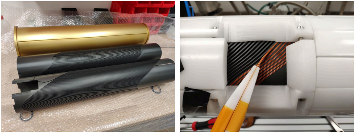
Figure 1. The hard-anodized aluminum formers and the winding test of the SuShi septum magnet prototype.
