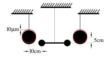
Figure : Schematic view of a Cavendish experiment where the delay  $au_{delay} \sim 1$ ms would shift the 5th digit of the measured G by -8.
