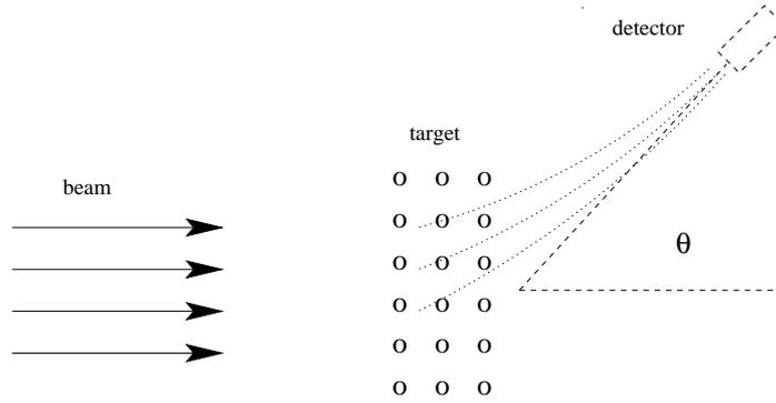
FIG. 18: Schematic view of a scattering experiment
